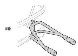
Release the axle and remove the Trailer Yoke
